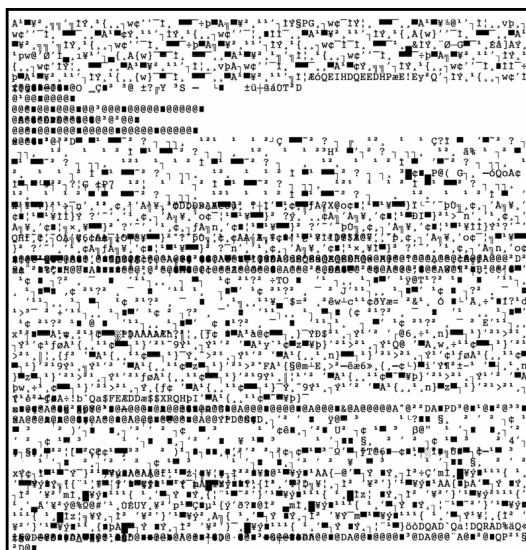
Printer Test Page printed with the incorrect page description language or incorrect driver
