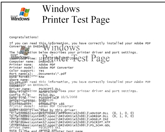
A "ghosting" Windows Printer Test Page from a laser printer with a faulty cleaning subsystem
